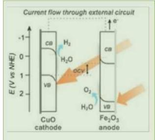
Figure 4: The operating principle of the planned hybrid tandem photoelectrochemical system
