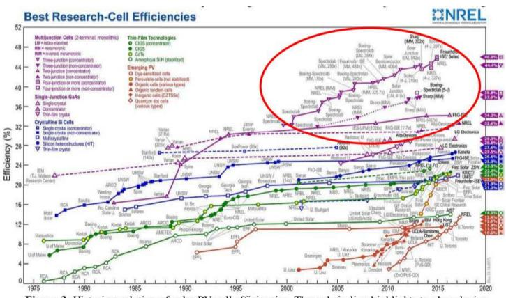
Figure 3: Historic evolution of solar PV cell efficiencies. The red circling highlights tandem device architectures, which are the highest performing (source: National Renewable Energies Lab, USA)
